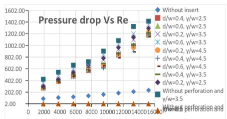
Graph 7 Effect of Pressure Drop over the Reynold's Number for different arrangement
