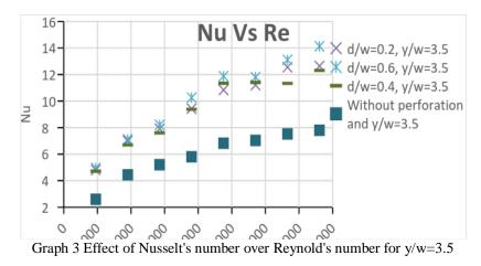
Considering the effect of twist ratio on Nusselt number it is found that with increase in y/w up to certain condition along with d/w the values is going to increase and letter on it will get decrease. This is because of the turbulence intensity generated in fluid.
