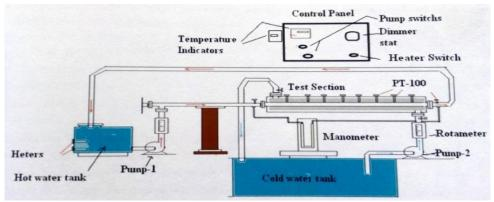
Figure 1 Schematic diagram of experimental Setup
